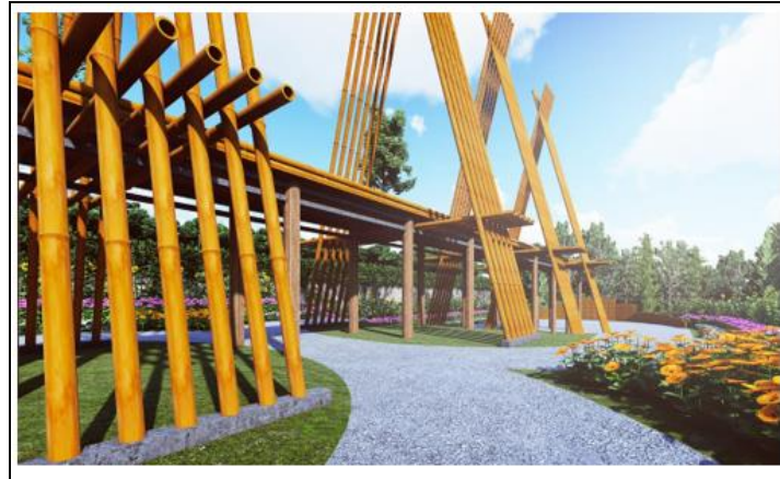
Figure 8: Bamboo material considers availability, low carbon footprint, and culturally relevant construction techniques.
