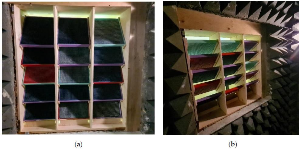
Figure 7. Tire rubber as a waste-based material, (a) tilted towards the noise source, (b) tilted away from the noise source Source: Strazdas & Januševičius, 2024
