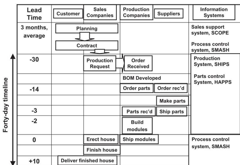
**Figure 5** Typical prefabrication schedule of Sekisui House (Source: Atkinson, 1999)
