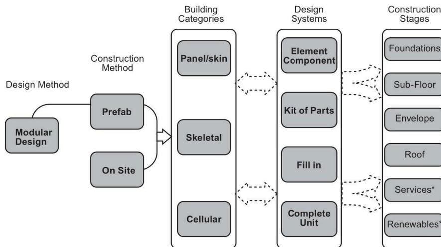
**Figure 1** Categorization of prefabricated systems
