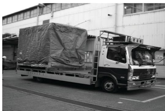
**Figure 12** Transporting a volumetric module of Sekisui House
