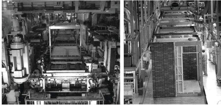
**Figure 9 and 10** Volumetric module's production line in Sekisui House
