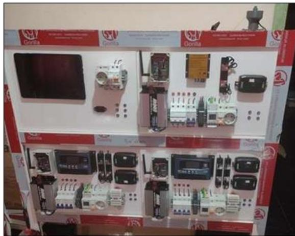
**Gambar 3.** Alat sistem monitoring PLTS berbasis *Smartphone*
