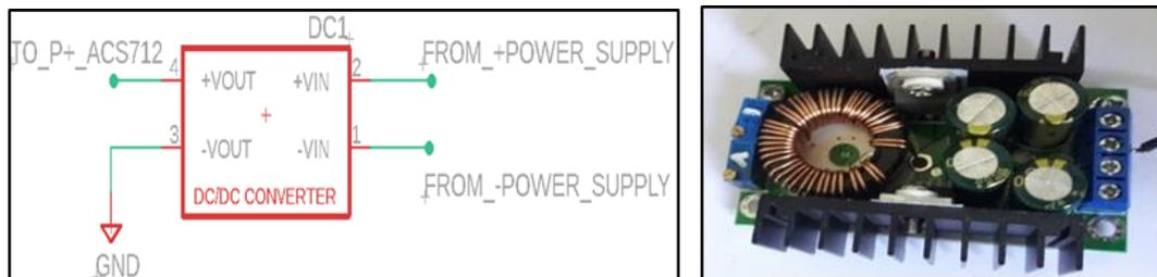
Gambar 2.3. Rangkaian DC to DC Converter Module
