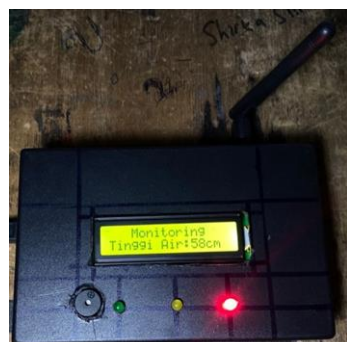
Fig 10. Displays a warning condition because the water level is > 45 cm
