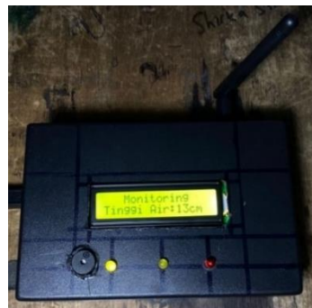
Fig 8. Displays a safe condition because the water level is < 25 cm
