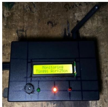
Fig 9. Displays an alert condition because the water level is 25 cm
