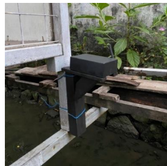
Fig 8. Displays a safe condition because the water level is < 25 cm
