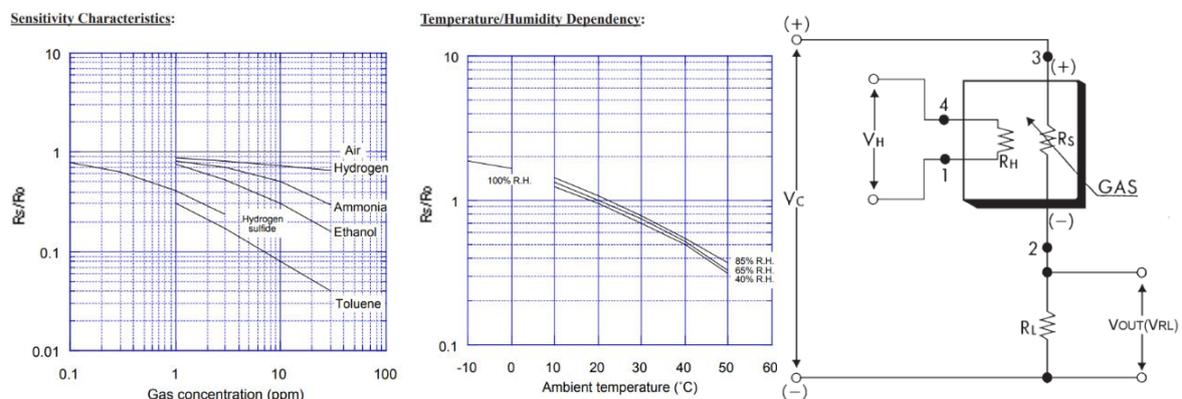
Fig 1. Sensor Characteristic Graph [12](left), Basic Circuit [12](right)
