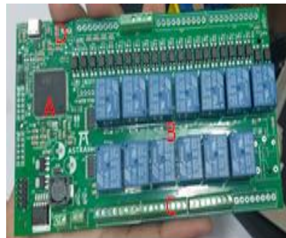
Fig 3. Electronics Board (a) Microcontroller, (b) Relay block, (c) Input/Output, (d) USB connector
