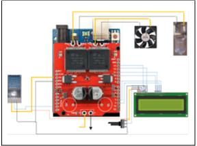
Fig. 1. Arduino Uno pin connection with other device
