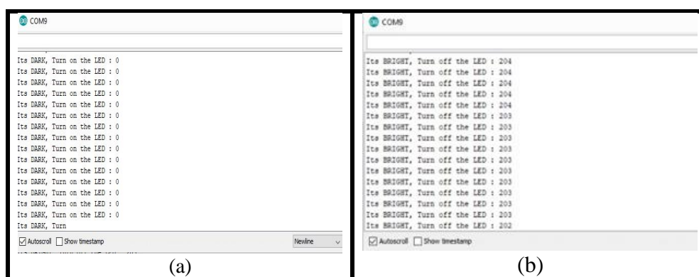
Fig. 2. (a) Serial Print LDR sensor readings when it's not detecting movement, (b) Serial Print LDR sensor readings when it's detecting movement
