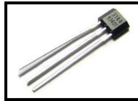
Fig. 2. Sensor Hall Effect A3144
