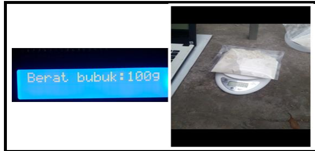
Fig. 14. Loadcell Weighing Results on LCD and Digital Scales (Weight 100 Grams)
