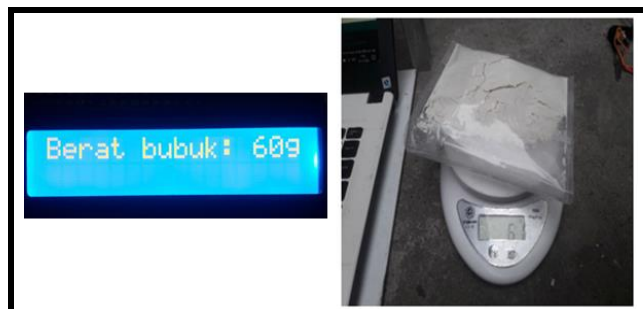
Fig. 12. Loadcell Weighing Results on LCD and Digital Scales (Weight 60 Grams)
