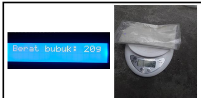
Fig. 10. Loadcell Weighing Result on LCD and Digital Scales (Weight 20 Grams)
