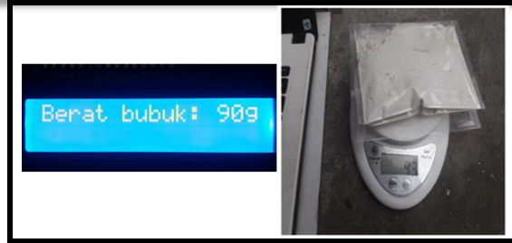
Fig. 13. Loadcell Weighing Results on LCD and Digital Scales (Weight 90 Grams)
