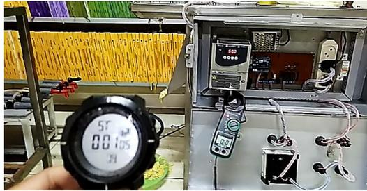
**Fig.23** Time of chopping at a speed of 260,1 Rpm
