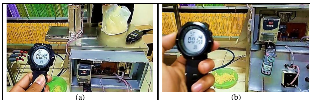
Fig. 5. (a) Time of chopping at a speed of 147,8 Rpm, (b) Time of chopping at a speed of 221,2 Rpm
