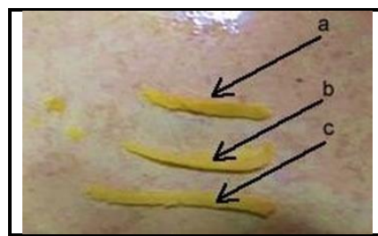
Fig. 3. Rebung Raised Results Based on VFD Settings (a) 50 Hz Frequency, (b) 35 Hz Frequency, (c) 20 Hz Frequency
