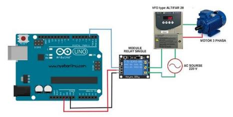
Fig. 13 Motor Control Circuit using VFD with Arduino
