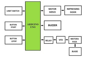
Fig. 6 Block Diagram Rebung Chopper Tool
