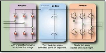
Fig. 1 Working of VFD<sup>[6]</sup>
