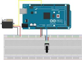
Fig. 11 Servo Motor Design with Arduino
