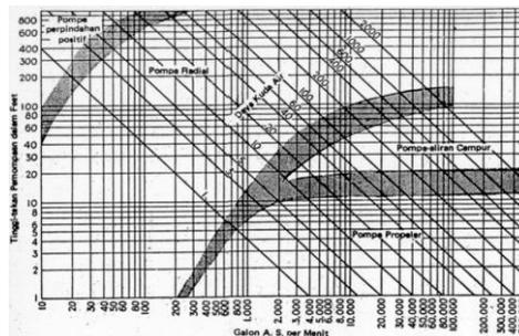
Figure 8. Pump selection diagram (Munson et al., 2002)
