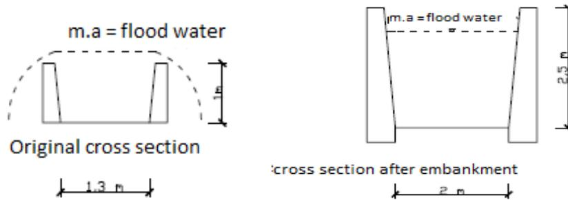
Figure 8. Original cross section
