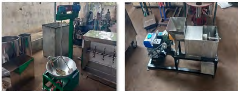
Figure 7. Trial of Jenang processing machine and coconut husks pressing machine
