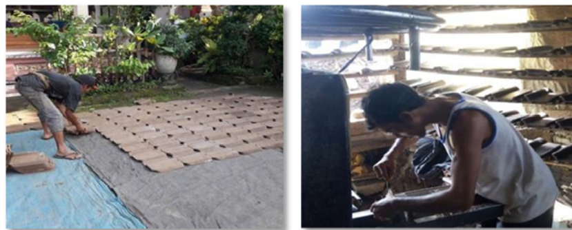
Figure 1. Manual production and drying process of traditional roof tiles
