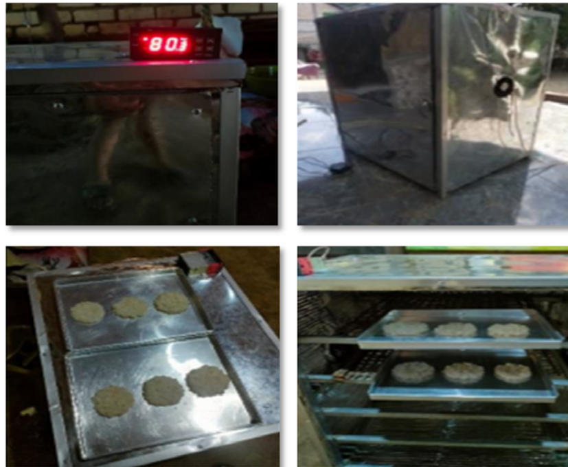
Figure 6. Implementation of the microcontroller-based food dehydrator for rengginang crackers
