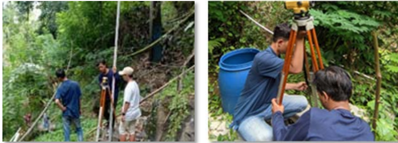
Figure 2. Elevation measurement using autolevel
