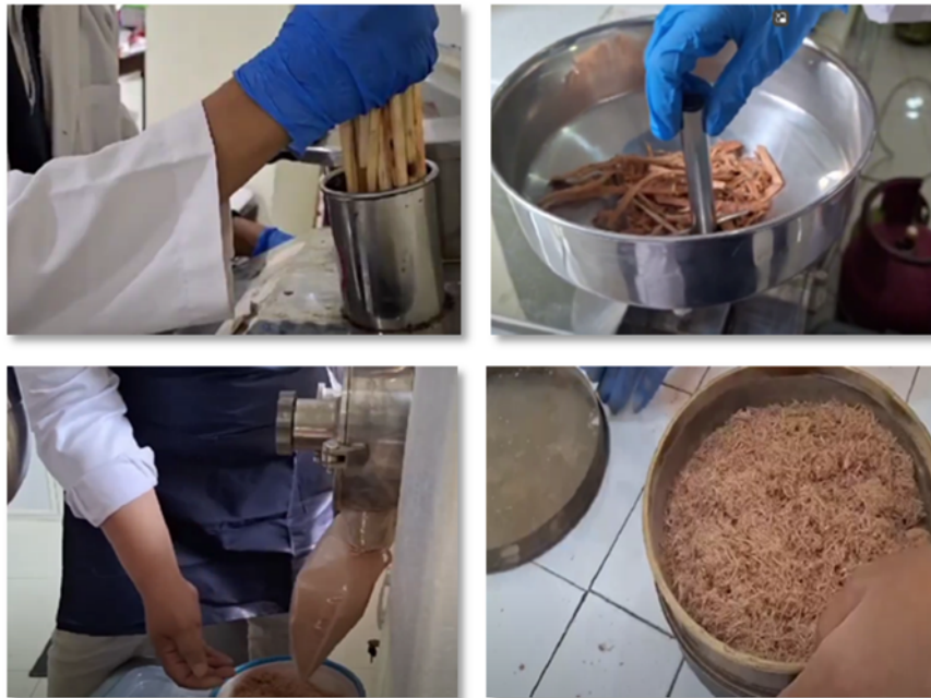
Figure 4. Grinding process with a disc mill into flour
