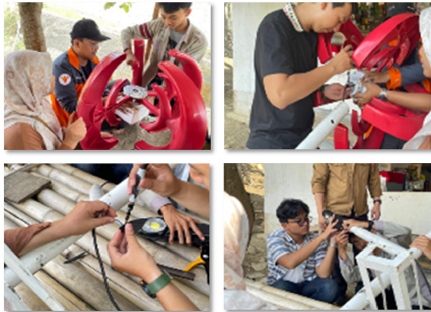
Figure 8. (a) Blade installation; (b) Blade assembly with rotor and generator; (c) Lamp cable assembly; (d) Lamp assembly with VAWT
