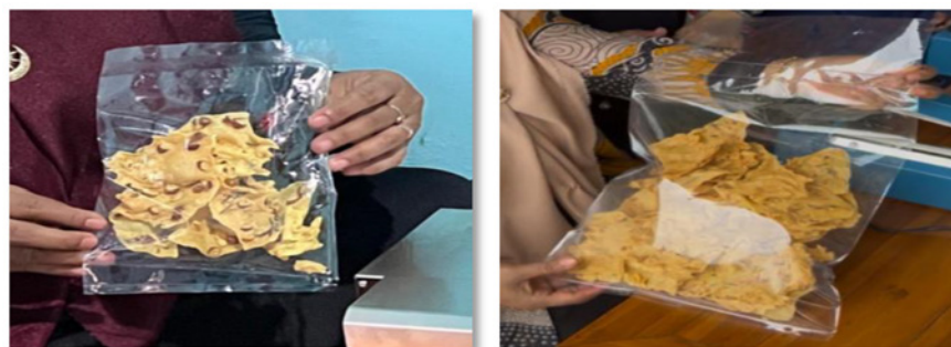
Figure 8. Packaging results of peyek products with continuous band sealer (left) and manual sealer (right)
