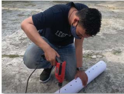
Figure 1. How to make a hole in the pipe
