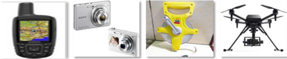
Figure 7. Equipment for surveying infrastructure and area boundaries: (a) GPS; (b) Digital camera; (c) Meter; (d) Drone
