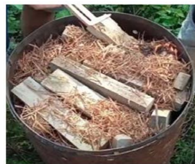
Figure 9. Inner and outer tubes of casting and filling of biomass for the casting process
