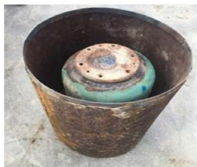
Figure 9. Inner and outer tubes of casting and filling of biomass for the casting process
