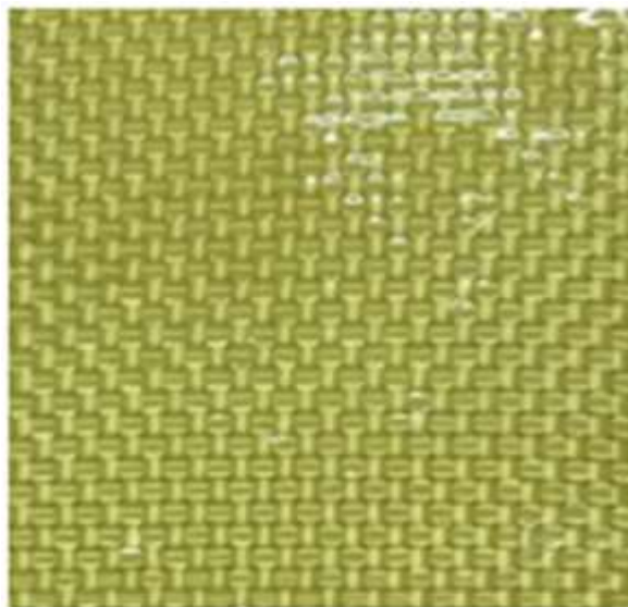
Figure 1. Kevlar with STF coated
