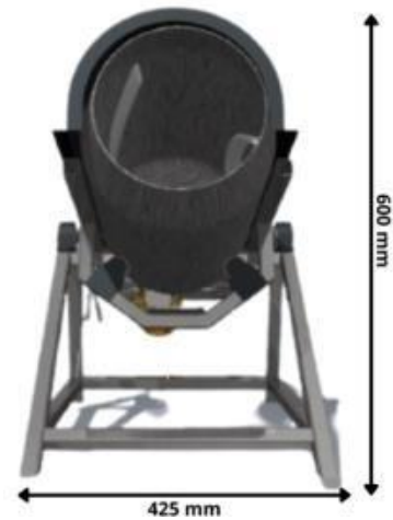
Figure 3. Coffee roasting machine with a horizontal cylinder with a capacity of 5 kg, front view
