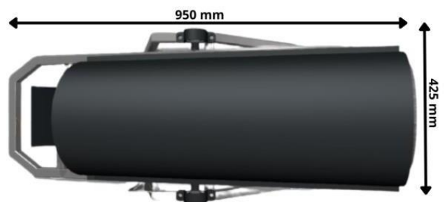
Figure 4. Coffee roasting machine with a horizontal cylinder with a capacity of 5 kg, top view
