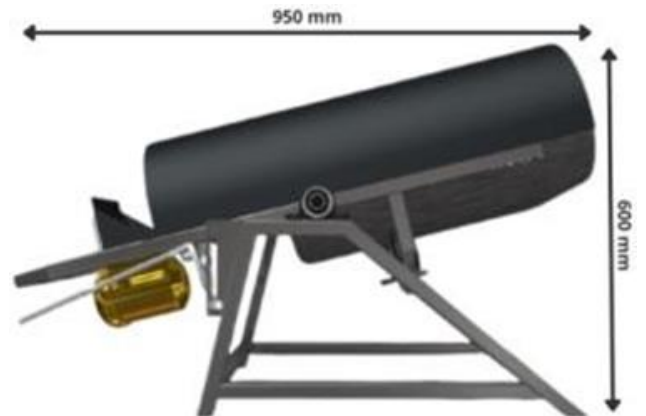
Figure 2. Coffee roasting machine with a horizontal cylinder with a capacity of 5 kg, side view
