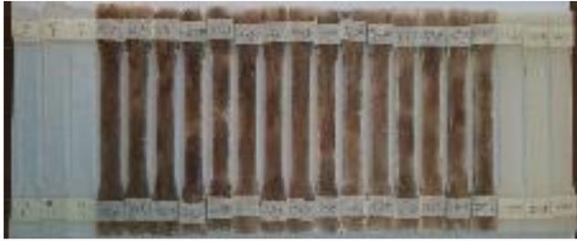
**Figure 3.** CaCO<sub>3</sub>/kenaf/epoxy composite specimen of tensile test
