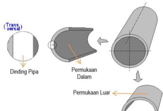
Figure 2. Specimen cutting
