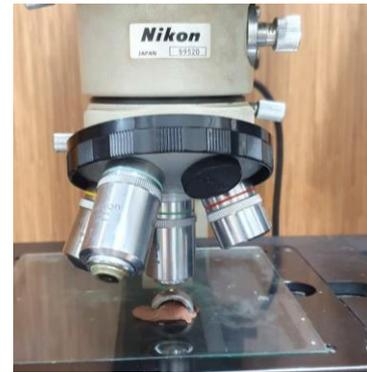
Figure 4. Observation of microstructure using a metallurgical microscope
