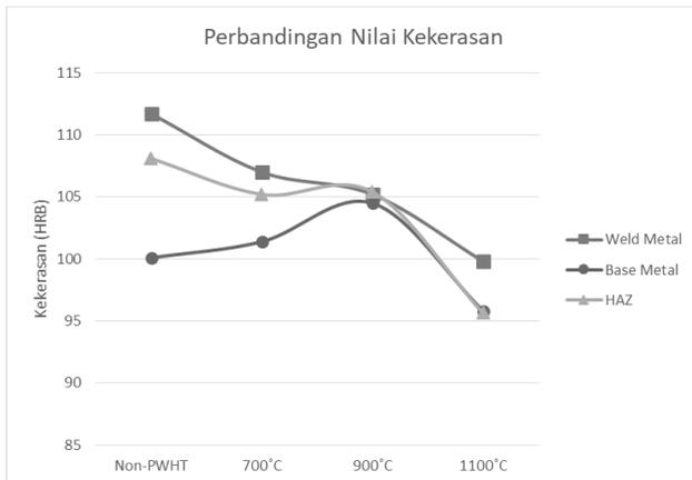
**Figure 13.** Comparison chart of hardness and PWHT process
