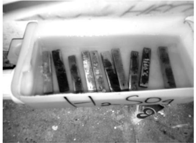
**Figure 9.** Immersion of Specimens in H<sub>2</sub>SO<sub>4</sub>
