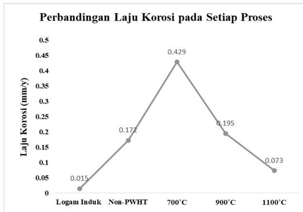
**Figure 14.** Corrosion rate comparison chart
