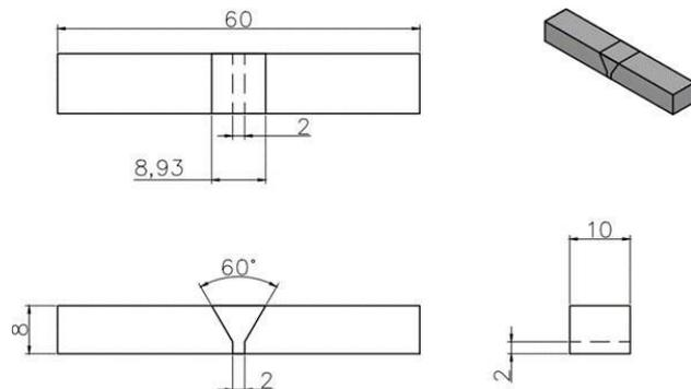
**Figure 5.** Technical drawing of specimen samples
