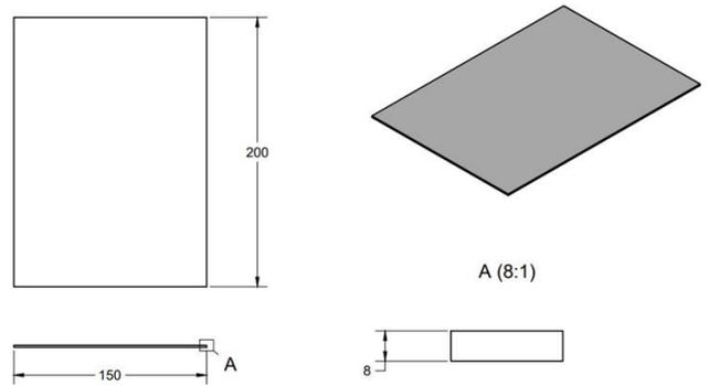
**Figure 2.** Material dimensions (AISI 304)
