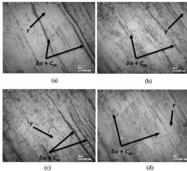
**Figure 11.** Microstructure in the HAZ Region (a) Without PWHT, (b) PWHT 700°C, (c) PWHT 900°C, (d) PWHT 1100°C.
