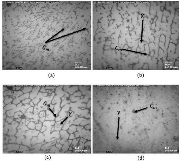
**Figure 12.** Microstructure in the Weld Metal Area (a) Without PWHT, (b) PWHT 700°C, (c) PWHT 900°C, (d) PWHT 1100°C.
