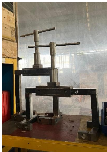
Figure 2. Flipper molding tool that has been fabricated
