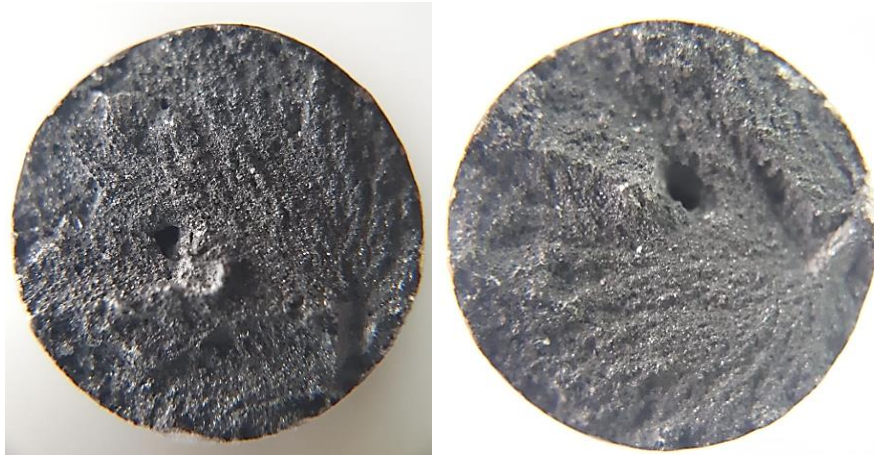
Figure 5. Macro Photo of Al-Si Fracture Temperature 600°C
