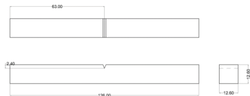
Figure 4 Impact test specimen ASTM D6110
