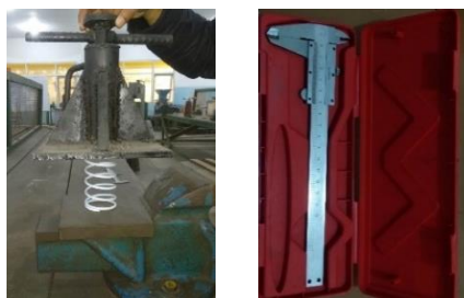
Figure 21. (a) Manual secondary spring testing (b) Vernier caliper
