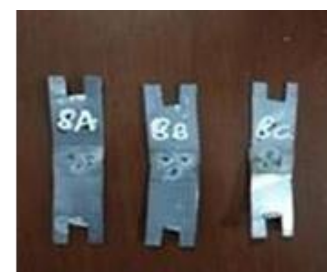
Figure 9 Spot Welding Result with 8-Second Weld Time
