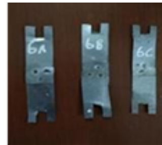
Figure 8 Spot Welding Result with 6-Second Weld Time
