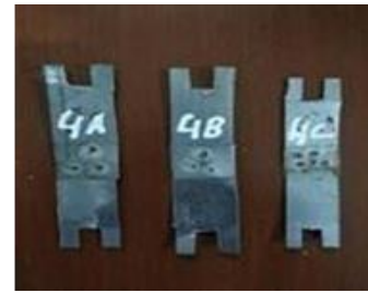
Figure 7 Welding Result at 4 Seconds
