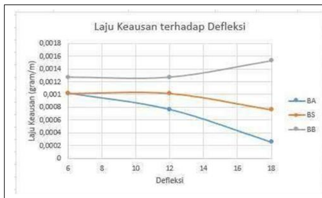
Graph 4.2. Graph of Wear Values for Square Profile Hollow Steel against Deflection Variations
