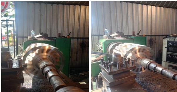
Figure 7. Vane Geometry Restoration through Reshaping
