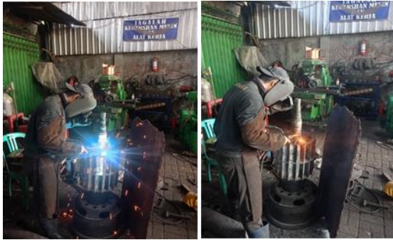
Figure 6. Weld Build-Up Process on the Vanes
