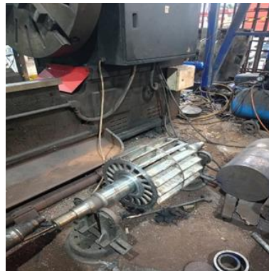
Figure 12. Impeller After Repair
