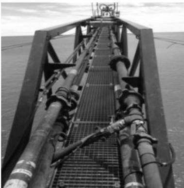
Gambar 1. *Boom Burner*
