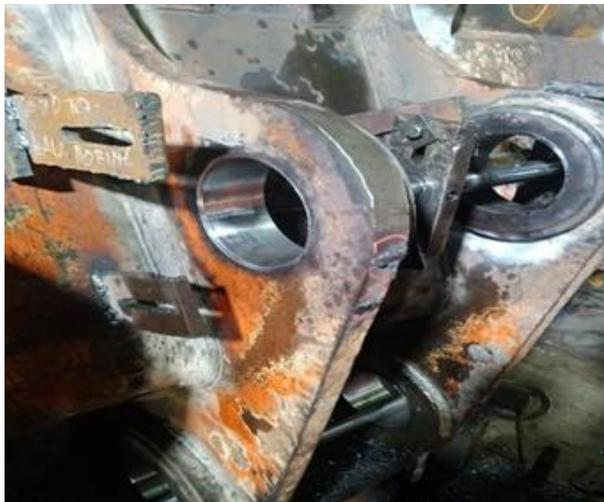
**Gambar 3** Proses melepas bracket liner boring
