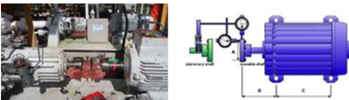
Figure 10. Shaft misalignment calculation
