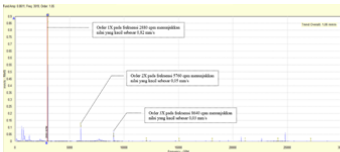
Figure 5. Motor vibration spectrum (alignment)
