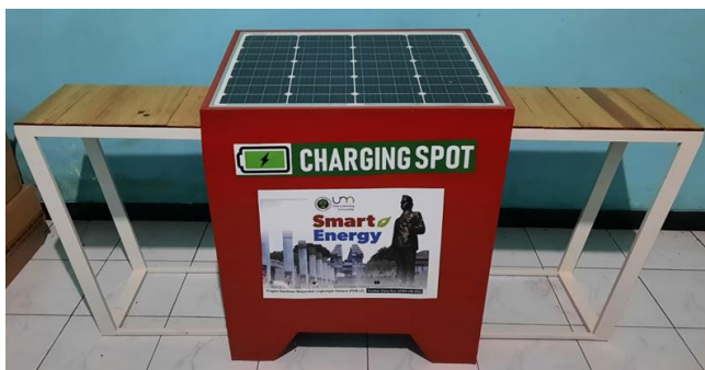
Figure 4 Solar Cell-Based Charging Spot integrated with Trash
