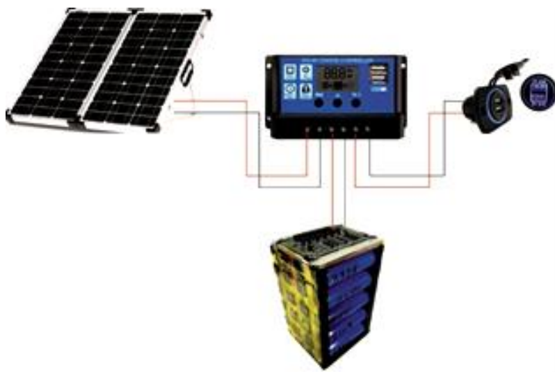
Figure 3 Solar Cell Based Spot Charging Design
