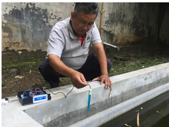
Figure 4. Application of Automatic pH Controller in One of the Tilapia Aquaculture Freshwater Ponds
