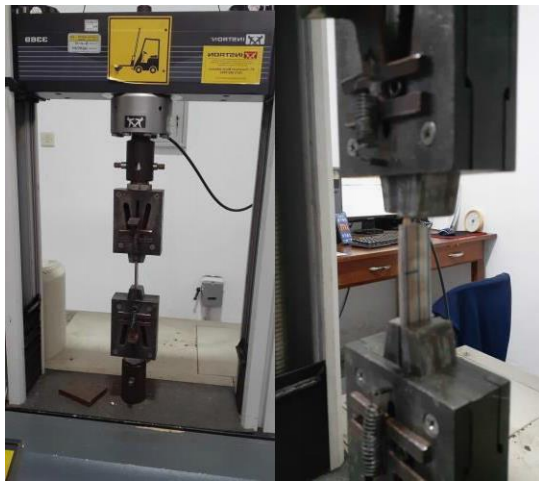
Figure 4. Universal Testing INSTRON Serial 3369
