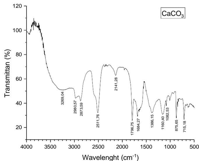
Figure 4. Analysis Results of FTIR Test on  $\text{CaCO}_3$
