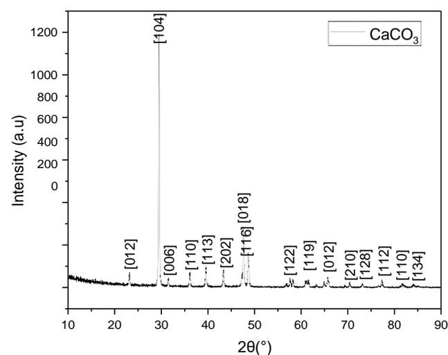
**Figure 3.** Graphic of XRD Test on  $\text{CaCO}_3$
