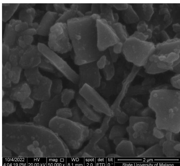
**Figure 2.** SEM Results on Calcium Carbonate ( $\text{CaCO}_3$ ) Nanoparticle with 50,000 Times Magnification
