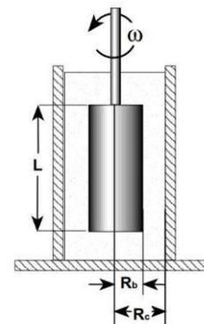
Figure 1. Spindles and Vessels for Rheological Measurements
