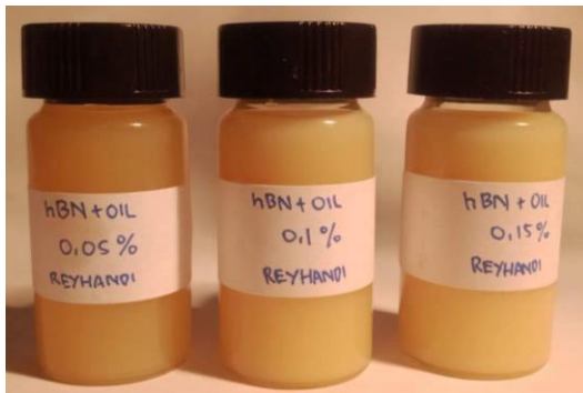
Figure 2. Results of Nanolubricant Preparation with Volume Fractions of 0.05, 0.10, and 0.15%
