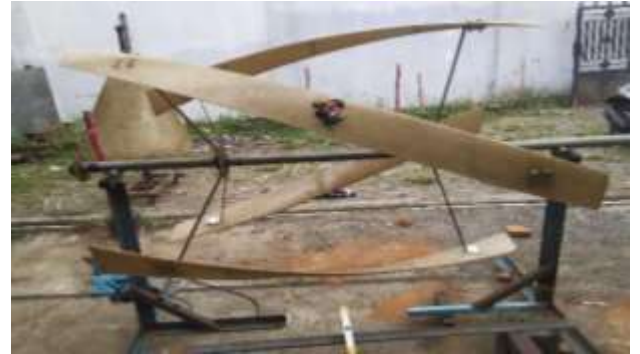
Figure 9. Balancing test with ballast on Helix blades
