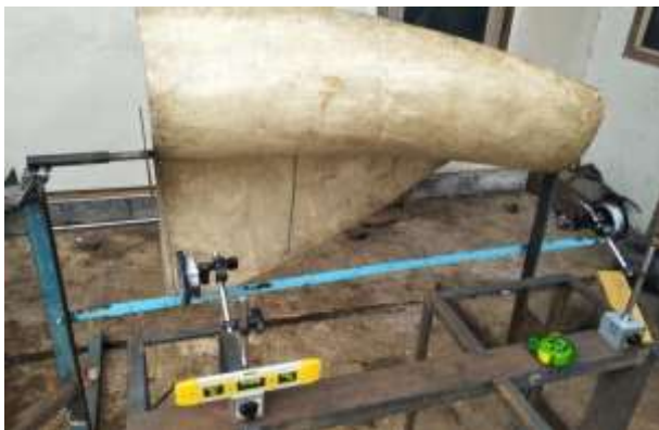
Figure 11. Savonius turbine blade alignment test
